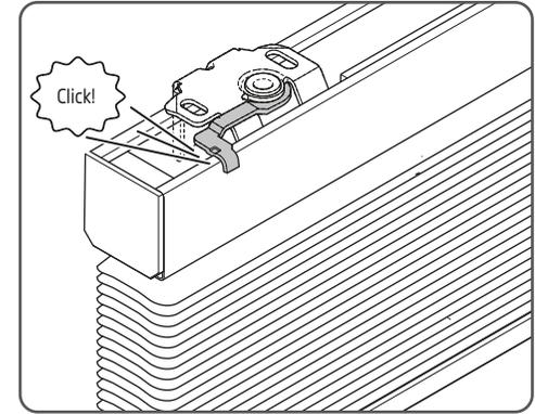
**!** Install the child safety as specified in the childsafe device manual.
